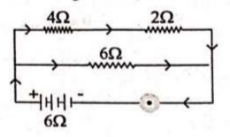
Calculate: (a) Total effective resistance. (b) Potential difference across  $4\Omega$ ,  $2\Omega$ .
